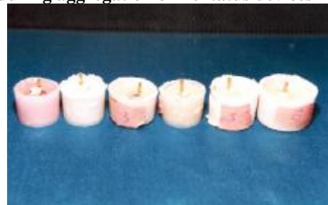
Figure no. 5. Lot of teeth prepared for determination of stress during aggregation of Dentatus devices
