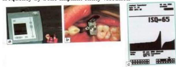
Figure no. 6. "Shock resistance" measurement of the bone-implant entity with the help of Osstell. Analysis of resonance frequency by bone-implant entity vibration
