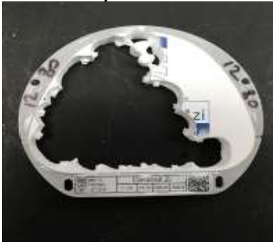
Figure no. 9. Dyeing of zirconium oxide before sintering
